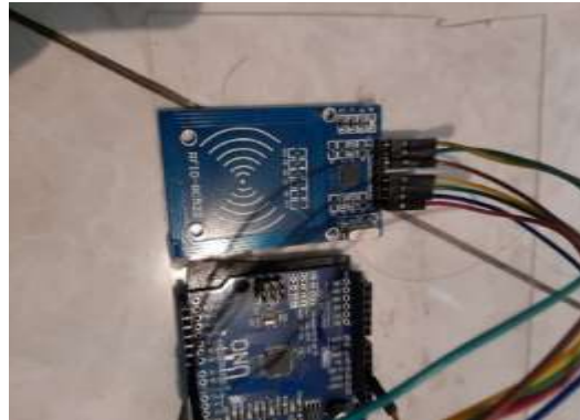
Figure 8. RC522 RFID Circuit
