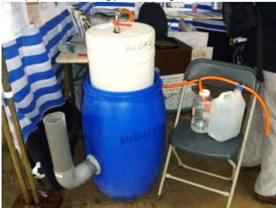
Figure 2: Collector Tank of Lab-Scale Biogas Reactor with Water Displacement Method for Biogas Measurement..
