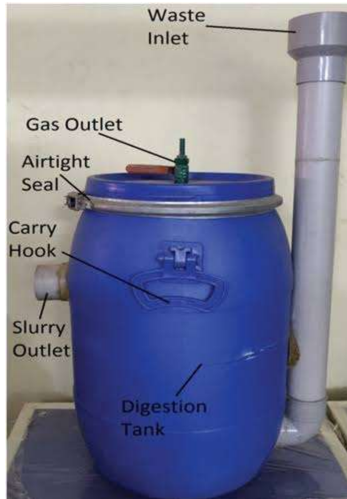
Figure 3: Digestion Tank Component of biogas Reactor.
